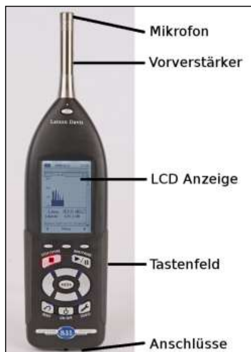
Abbildung 1.1: LD 831 (Anschlüsse, Tastatur, LCD-Display,
